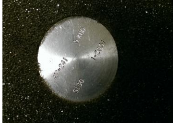
Figure 2 – Radioactive Source: Americium 241
